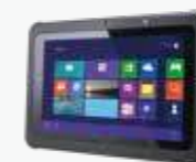
CAXA0 10.1" Semi-Rugged Tablet Intel Celeron N3350 MIL-STD-810G & IP65 certified
